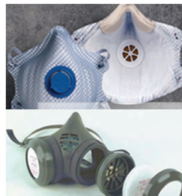
NIOSH-approved N95 filtering facepiece (top) and elastomeric (bottom) half-face respirators can be used only if silica concentrations are less than 10 times the PEL.
